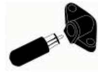
12V caravan socket & plug One pin. Polarised
